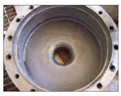
Infiltration Brazed Tungsten Carbide Cladding
